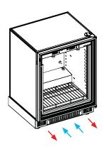
The air flows must not be mixed. Make sure that the incoming ai flow comes from outside by isolating the air flows. (By using adhesive foam for example)
